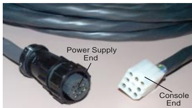
2600-18 PS Cable Pinout
